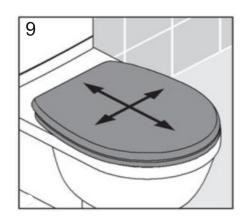
Adjust the Seat Cover by gently moving, by hand only, left and right, to perfectly fit with commode profile. Then fully tighten the wing nut (no.8) by hand only and Screw (no.1) by Star Screw driver.
