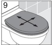
Adjust the Seat Cover by gently moving , by hand only, left and right, to perfectly fit with commode profile. Then fully tighten the screw ( no.3 ) by Star Screw driver.
